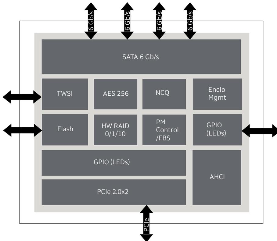
Fig 1. Block Diagram for Marvell 88SE9230
