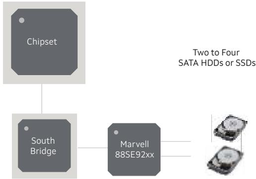
Fig 2. RAID-On-Motherboard Application
