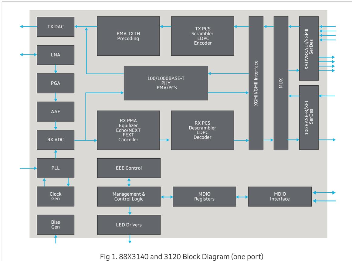
Fig 1. 88X3140 and 3120 Block Diagram (one port)
