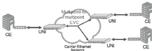
**Figure 4. Ethernet Private LAN (EP-LAN): port-based all-to-one bundling**
