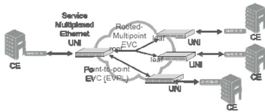
Figure 7. Ethernet Virtual Private Tree (EVP-Tree): VLAN-based service multiplexing
