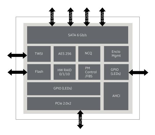
Fig 1. Block Diagram for Marvell 88SE9230
