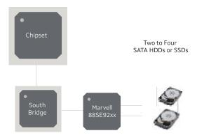
Fig 2. RAID-On-Motherboard Application
