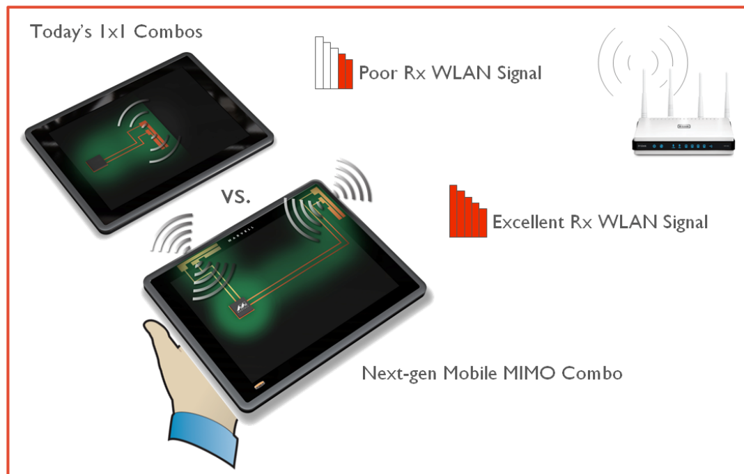
Figure 1: Mobile MIMO configuration with flexible antenna placement options reduce the likelihood of signal obstruction (i.e. user's hand)
