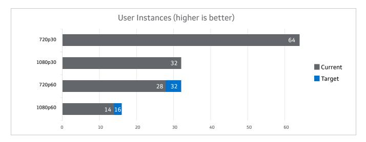
Using a single ThunderX2 server, with two GPUs for hardware rendering, Marvell's Android Cloud Gaming solution enables 64 user instances running High-Definition games at 720p30. The same solution scales with higher resolution and framerates as well, achieving 32 user instances at 1080p30, 28 user instances at 720p60, or 14 user instances at 1080p60.8
