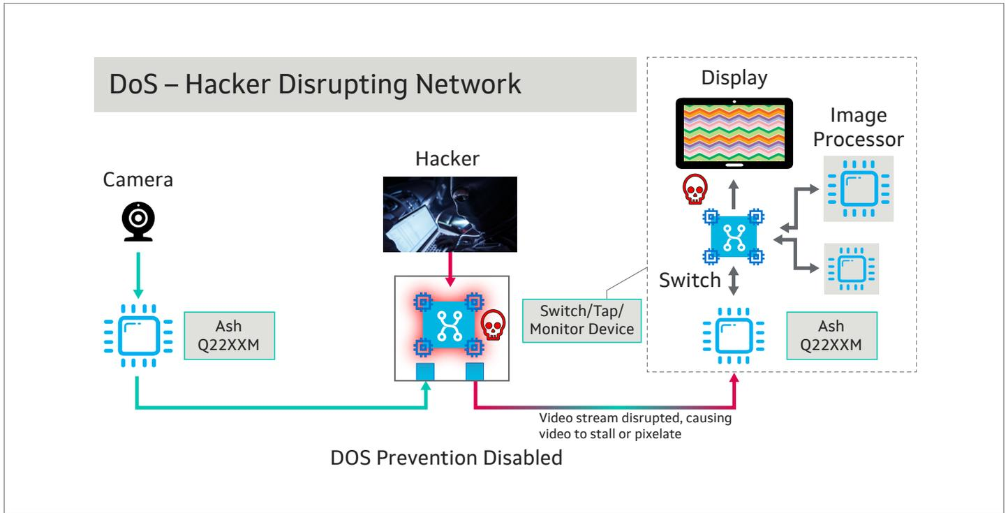
Figure 6e: Hacker executes Denial-Of-Service attack on the Image processing sub-system and jams the link.
