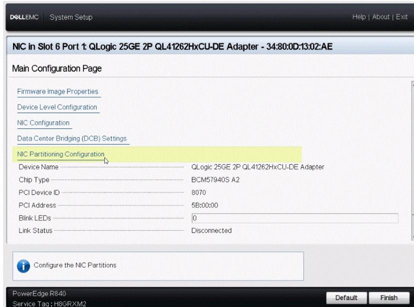
**Figure 1-8. Adapter Port Main Configuration Page**
