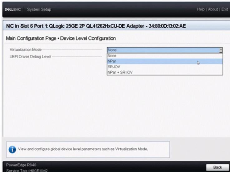
**Figure 1-6. Device Level Configuration Page**
