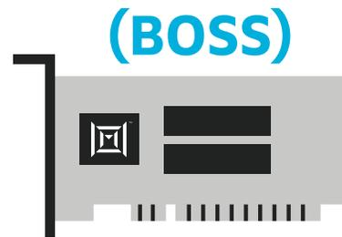
**MARVELL® M.2 BOSS card allows the server to boot the OS quickly and reliably using PCIe and M.2 RAID capable drives**
