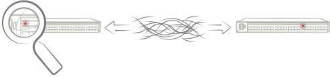
Figure 3: LCB Assists Operations When Attempting to Identify an End Point Link in a Large Storage Environment
