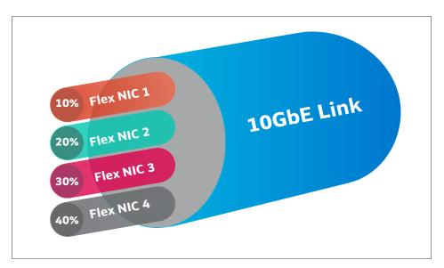
Figure 1. Physical Port Partitioned into Four Functions
