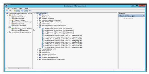
Figure 2. Windows Device Manager NPAR Enabled
