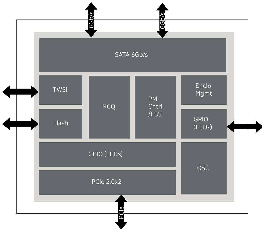
Fig 1. Block Diagram - 88SE9182 PCIe 2.0 to 2 Port 6Gbps SATA I/O Host Controller
