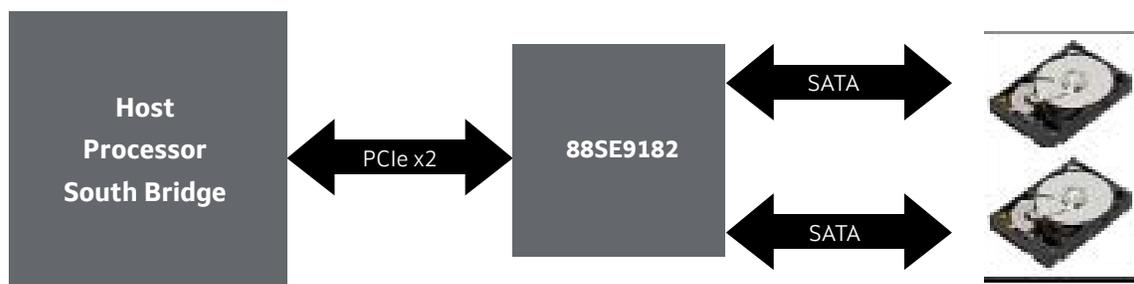
Fig 2. Typical Two Disk Application Example of 88SE9182
