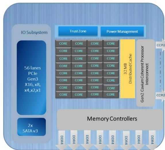
Figure 1: High Level Block Diagram of Marvell ThunderX2
